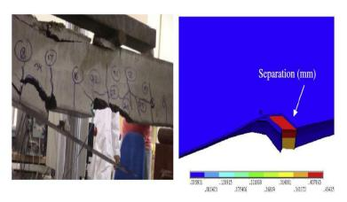
Fig 9 Simulated and Experimental Results of CFRP Plate De-Bonding
