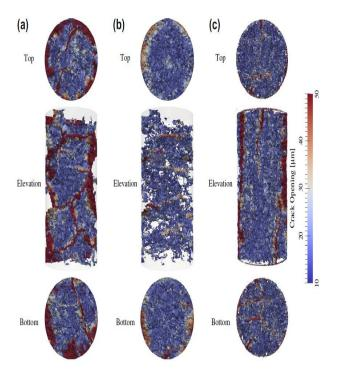
Fig 6 Crack Patterns Simulated In One Specimen For (a) Free Expansion Case, (b) 0 Mpa And 5-Mm-Restraint Case And (c) 20 Mpa Unrestrained Case
