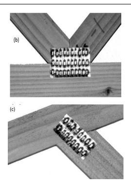
Fig 3 Model Truss Connections: (a) Peak Joint; (b) Bottom Chord Truss Joint; (c) Top Chord Web Joint
