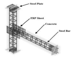
Fig. 11 Finite-element illustration of retrofitted specimen
